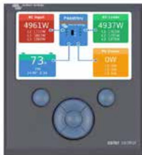
Color Control GX, showing a PV application
