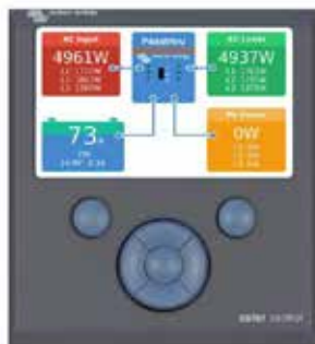
Color Control GX, showing a PV application
